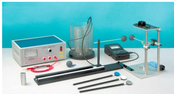
Figure 2: Coulomb balance equipment
